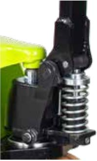
The Hydraulic pump is the core component of the hand pallet truck. The GS and GS EVO pump is designed and built in Italy with extreme care and attention to detail. This gives our pump the superior characteristics and features of:
