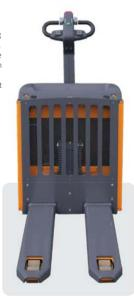
The OMG 316 KN-C ac combines the traditional function of the powered pallet truck (1.600 Kg capacity) to the possibility of lifting the load (1.000 kg capacity) up to 1.485 mm height from the ground. It can be used for picking and stacking operations. It is ideal to be used in warehouses with reduced distances and spaces and for the safely loading of overlapped loads.
