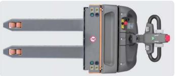
In the 316 KN-M ac the push buttons positioned in both sides are easily accessible for the operator who can better level the load acting on the lifting and lowering improving and limiting the pathologies related to the skeleton-muscle apparatus.
